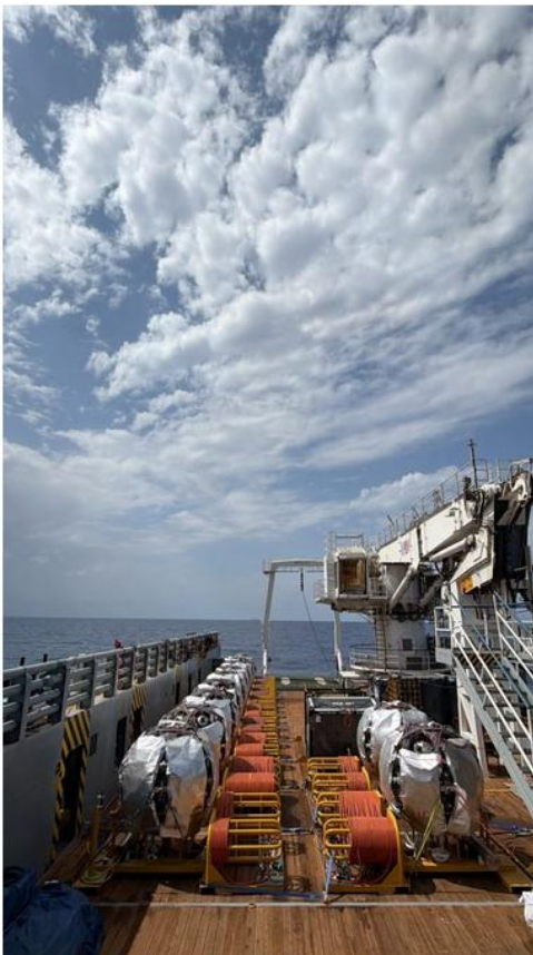
The deck of Ievoli Amber loaded with detection units awaiting deployment at the ARCA site.
