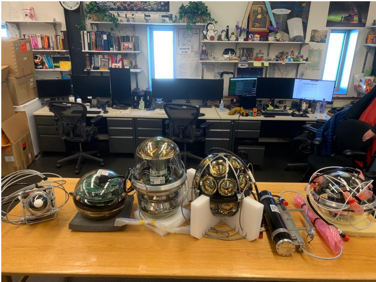
Credit: Sarah Mechbal, IceCube/NSF: DOMs and special devices, including the D-Egg (third from left) and mDOM (fourth from left), are on display in the science lab at the South Pole station.
