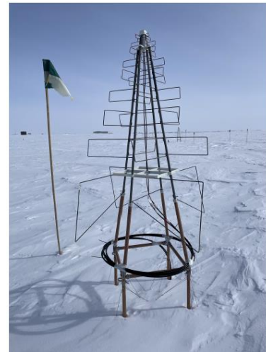
One of the three radio antennas of the prototype surface station at the South Pole (photo from December 2022)
