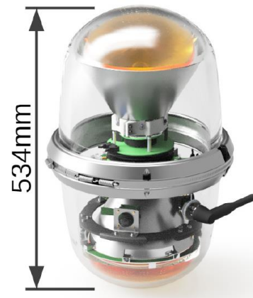
CAD rendering of an assembled D-Egg. The annular PCB comprising the LED calibration system can be seen resting in the optical gel gluing the lower PMT to the glass pressure vessel.
