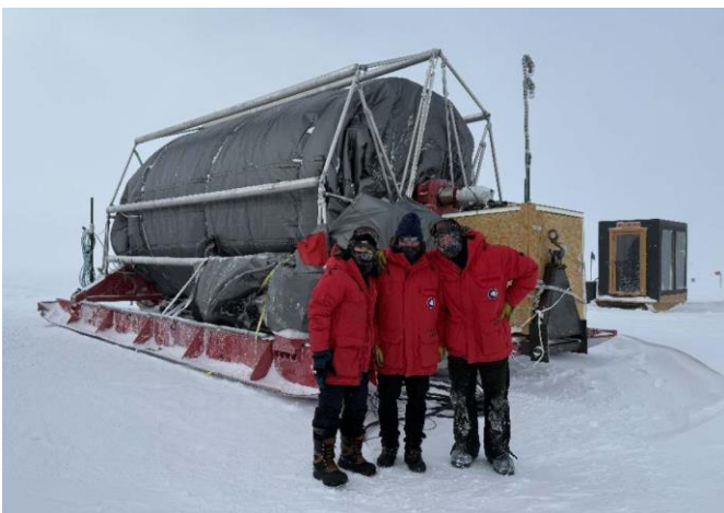
Members of the drill team with the heated drill hose. The drill must be heated to keep it at a tolerable temperature during the coming winter.
