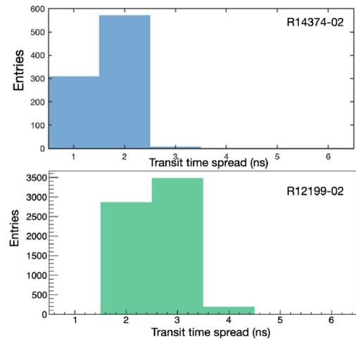
Measured transit time spread for a set of 1000 PMTs R14374-02 (top) and for the R12199-02 model (bottom).
