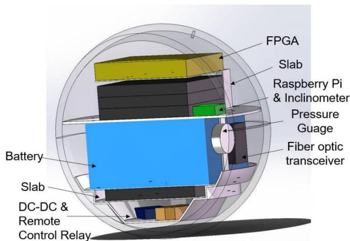
*Glass vessel and key ingredients of MuonSLab.*
