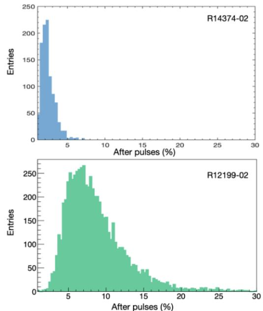
Measured rate of after pulses for a set of 1000 PMTs R14374-02 (top) and for the R12199-02 model (bottom).
