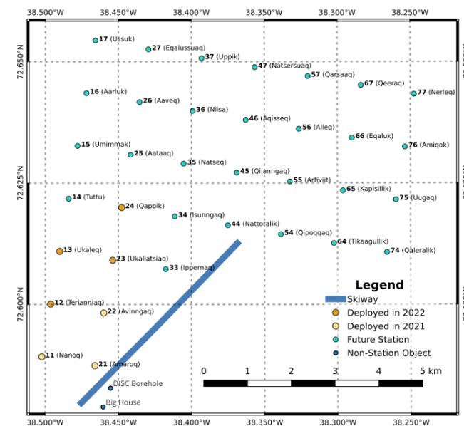
Planned and existing layout of the 35-station array of RNO-G. The first seven stations, the subject of this paper, were deployed in 2021 and 2022. The main building of Summit Station is labeled Big House.
