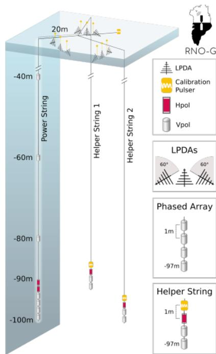
The station construction as installed for the first seven stations of RNO-G, showing the three instrumented boreholes down to 100 m, as well as the antennas in shallow trenches near the surface.
