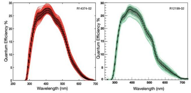
Photocathode quantum efficiency measurements as a function of the wavelength for 200 R14374-02 (left) and 46 R12199-02 (right). The improvement (from right to left) is relatively small.
