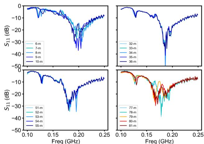
Measured S11 at various depths in ice. The anomalous response is highlighted, showing the abrupt change in the shape of the resonance. Note the relative constancy of the S11 shape in the depth interval from 32 to 55 m, in contrast to shallower depths and also the depth interval  $z \approx 80$  m.
