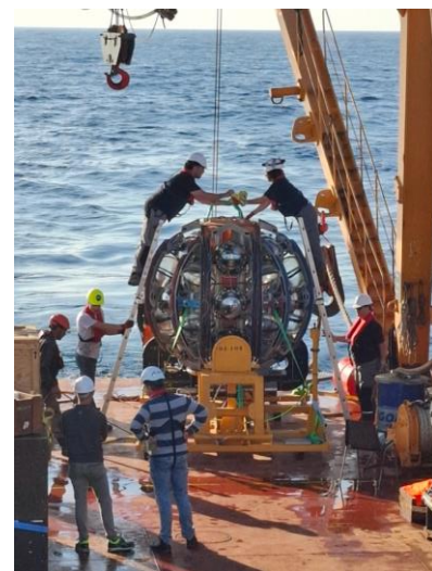
Preparing an ORCA DU for deployment
