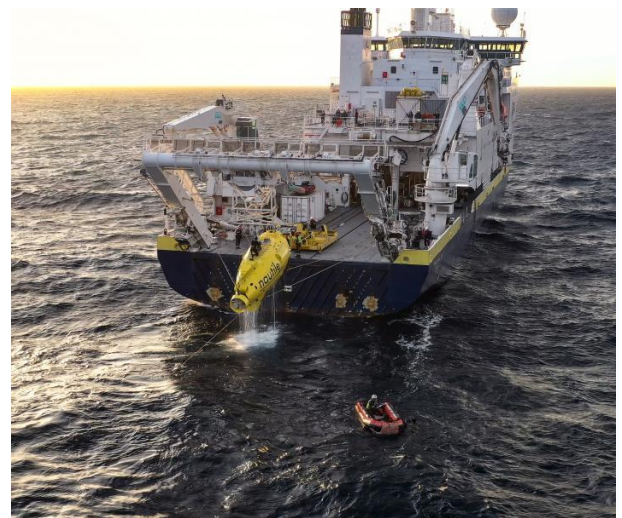
The Nautilie submarine on the Pourquoi pas?, used to connect the instrumentation to the scientific junction box.
