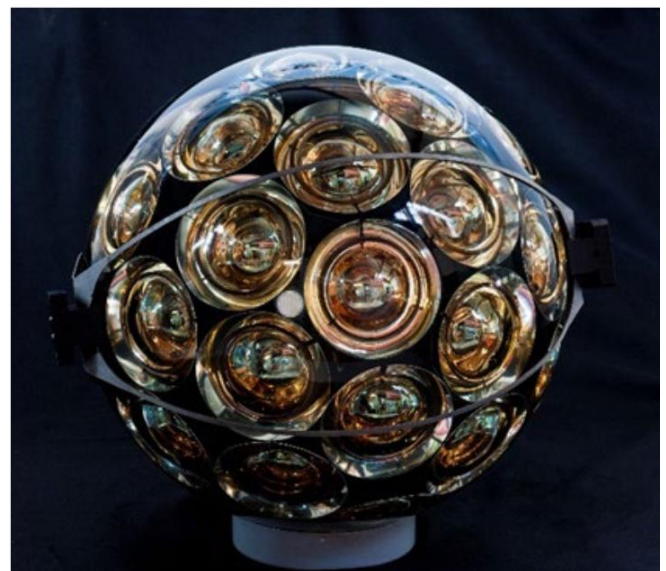
View of an optical module, illustrating its large effective and segmented photon detection area. On the left of the middle PMT, the acoustic piezo sensor used for positioning measurements is visible. The sphere hangs in a titanium collar required for mounting it along a detection unit ("string"). In this picture, the optical module is shown bottom-up.
